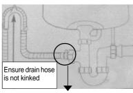
Remove blanking plug/closed end connection from sink trap.
